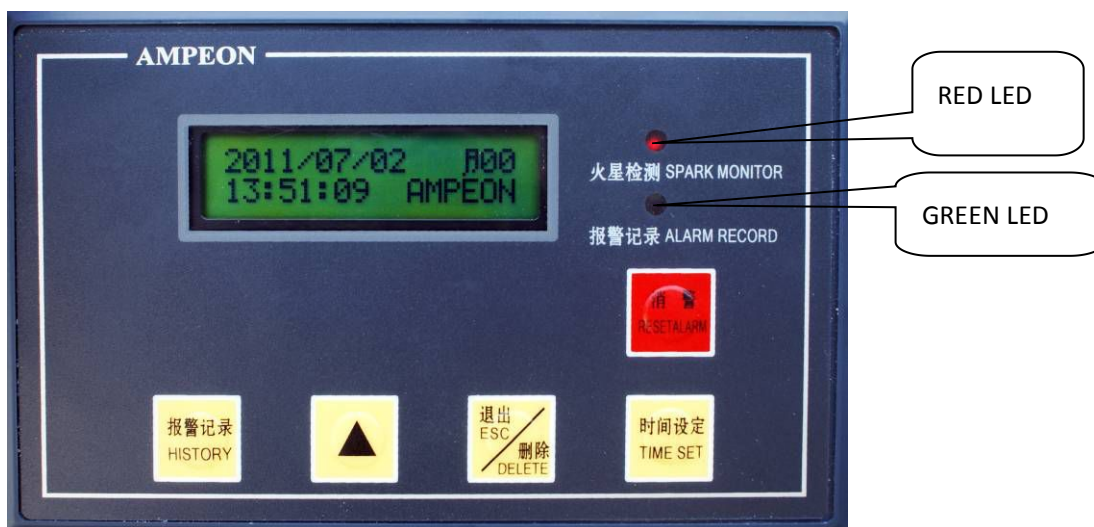
Figure 9: Control panel and main page
