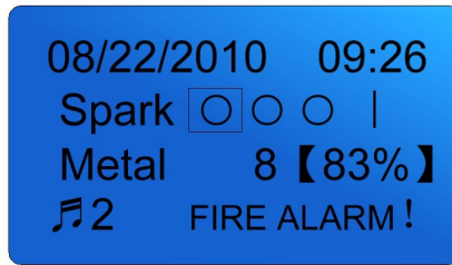
Figure 12: The fire alarm display
